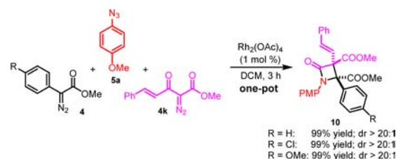
Scheme 4. One-Pot Multicomponent Synthesis of \beta -Lactam 10
